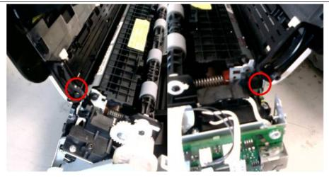
5. Remove the metal plate after unplugging the fuser connector.
