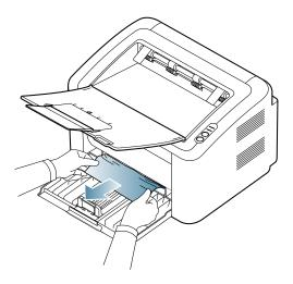
If the paper does not move when you pull, or if you do not see the paper in this area, check the fuser area around the toner cartridge.
