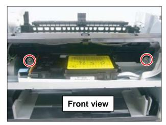
3. Remove 3 screws. Release the LSU.
