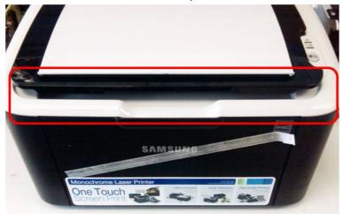
2. If the problem persists, check the cover open sensor that is located on the HVPS board.
