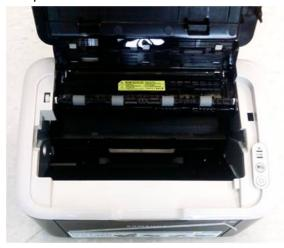
2. Reinstall the toner cartridge two or three times to confirm it is seated properly.
