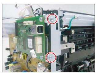
3. Remove 8 screws. Unplug a connector. And release the SMPS/HVPS board.
