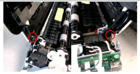
5. Remove the matal plate after unplugging the fuser connector.
