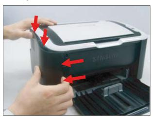
2. Take off the right cover by removing hooks from its edge.
