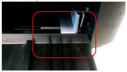
3. Check the maximum paper capacity of the tray. Remove excess paper from the tray.
