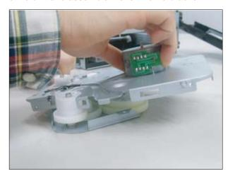
3. Remove 2 screws. Release the step motor.
