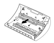
4. Remove PCB from the PCB cover.
