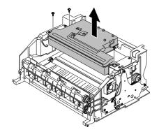
3. Remove two connectors from the LSU, then remove the LSU.
