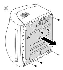
Unplug connectors from the main board and connectors from SMPS, then remove the SMPS. Remove four screws from SMPS and remove the SMPS board.
