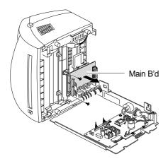
3. Release four snap-fits securing the insulator engine board and then remove the insulator.
