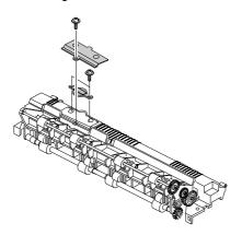
3. Take the halogen lamp out from the Heat Roller.
