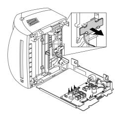
4. Release four snap-fits securing the sensor board and then remove the sensor board.
