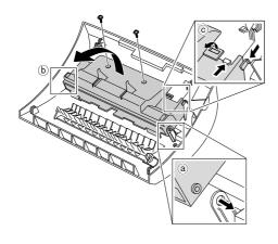
3. Remove two screws, and remove LED panel.
