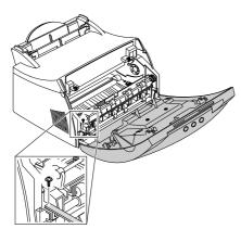
Loosen the right lower part of the cover, then push the cover in the direction of arrow to loosen the left lower part.
