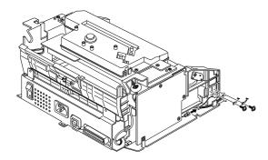
3. Remove two screws and unplug a fuser assembly harness. Then use a " - " screwdriver to unlatch the fuser assembly to remove.
